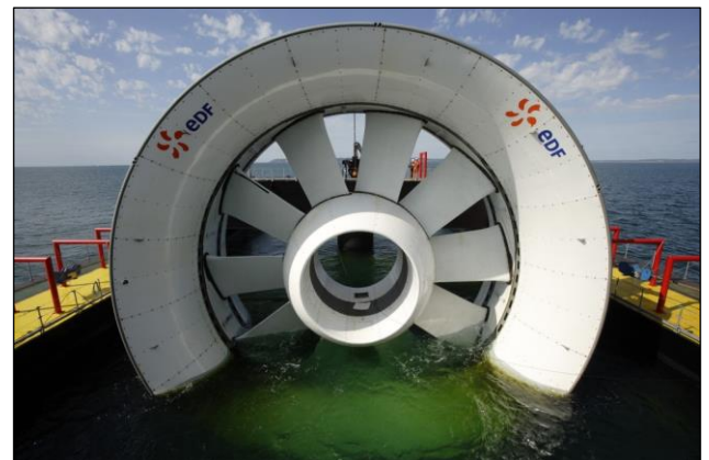
Fig. 5. Hydrolienne OpenHydro (500 kW).
