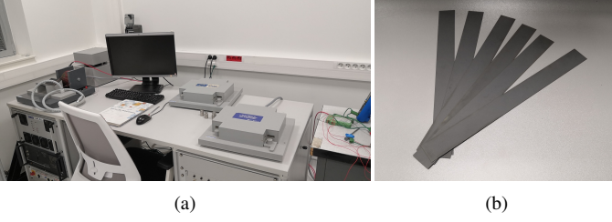
Figure 1. Measurement device: (a) Brockhaus MPG200D equipment and (b) Epstein samples
