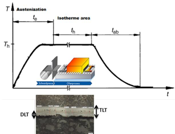
Figure 1: diagram of austenization
