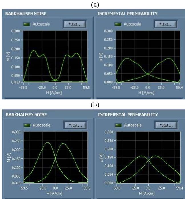
Fig. 3. BN and IP signals for coated hard and soft 22MnB5
