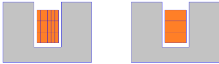
Fig. 6. Determination of the equivalent winding geometry when the six turns of each winding layer can be merged into one solid conductor
