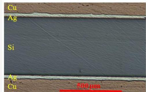
Figure 4: Cross-section of a 3D silver sintered assembly
