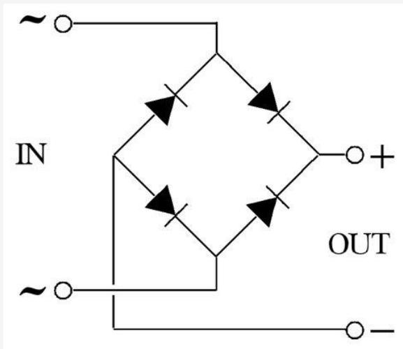
Figure 5: Bridge rectifier electric scheme
