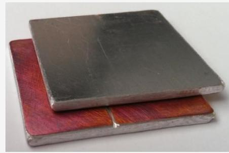
Figure 7: 3D silver sintered wireless bridge rectifier
