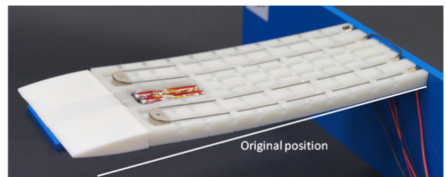
Fig. 1. Hybrid flap with both SMA and piezoelectric actuators
